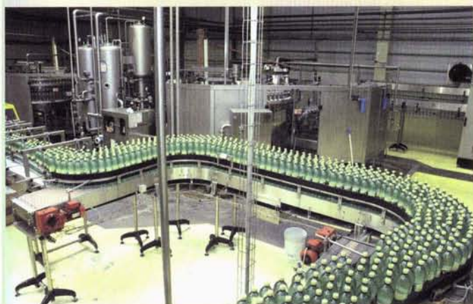
Mineral water and over 60 non-alcoholic refreshment beverages are filled in disposable PET bottles on two filling lines
